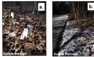
Fig. 2. (a) Close-up of two of the installed soil water samplers. (b) Samplers in nest B (see Fig. 3) that were installed 1.5 m away from the road. The white hue on the road is from a recent salt application.
